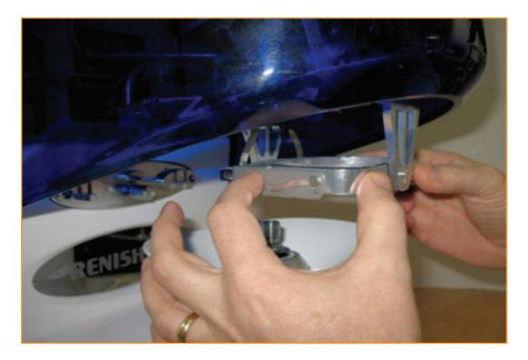
2. Push up the side arms and rotate them towards the front of the machine. The carrier tray will drop down to allow the billet to be inserted.
