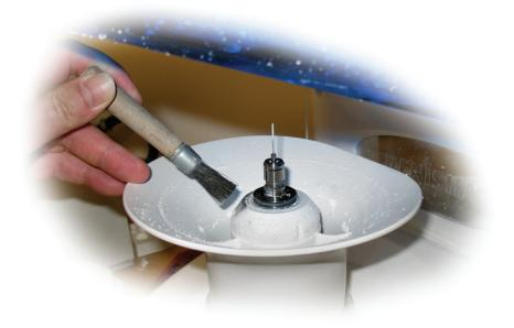
2. Remove the collet and tool holder. Clean the dust out of the collet and the spindle.
