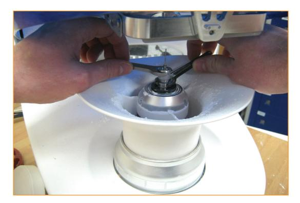
**IMPORTANT:** Do not tighten the collet nut until the tool is inserted.
