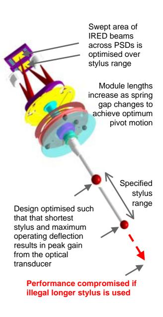
The **low probe mass** allows a low spring rate whilst retaining improved dynamic response over traditional scanning probe designs. The improved dynamics of **SP25M allows faster scanning measurements to be taken.**
