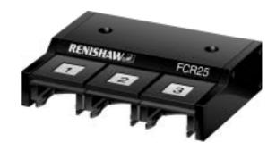
The ports in the FCR25 store the SM25-# and TM25-20 modules, but can quickly be configured to store the SH25-# stylus holders or TP20 modules by use of the appropriate port adaptor insert: PA25-SH (for SH25-#) or PA25-20 (for TP20).
