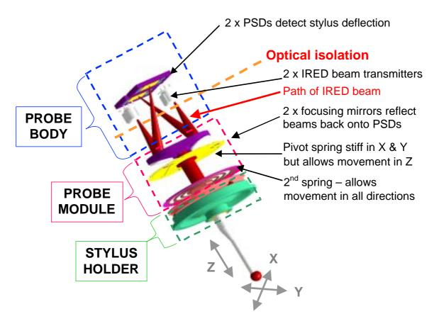
The pivoting motion system comprises **two diaphragm springs** and a **ferrofluid damping system**. One spring allows movement in all directions whilst the other (pivot) spring is stiff in (probe) X & Y but allows movement in Z. The reflective mirrors are integrally mounted to the motion system and therefore move directly with stylus deflection.
