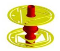
The patented, pivoting motion system features two diaphragm springs. One spring allows movement in all directions whilst the other (pivot) spring is stiff in (probe) X & Y but allows movement in Z. The three scanning modules are of different lengths to accommodate the optimised positioning of, and pitch between, the spring arrangement. This will be explained in more detail in 'key innovations' below.
