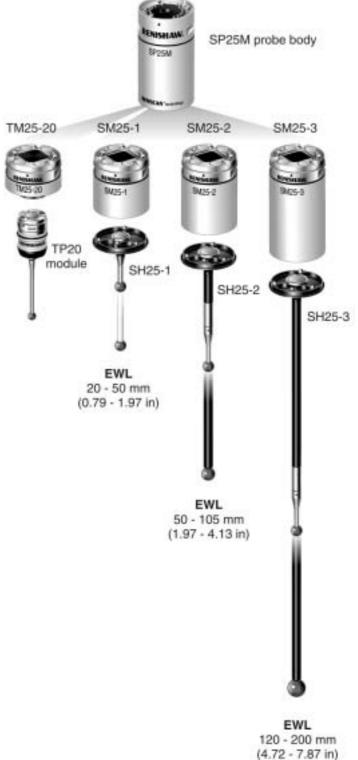
The joints between the elements are highly repeatable, thus eliminating the need to re-qualify (re-calibrate) after interchange. They work on proven kinematic location principles with simple magnetic attraction.
