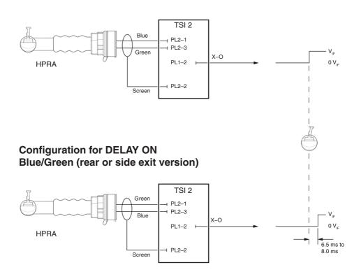
**NOTE:** Probe trigger delay is only compatible with on-centre length measurement; it should not be used for setting the ROTATING DIAMETER.
