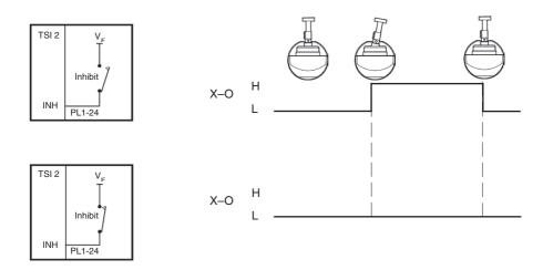
NOTE: The probe status LED will still function when inhibit is active.
