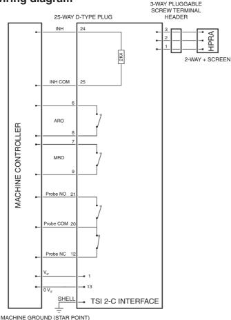
$V_{IE} = 24 \text{ Vdc PELV } 0.75 \text{ to } 1.25 \times \text{rated voltage.}$
