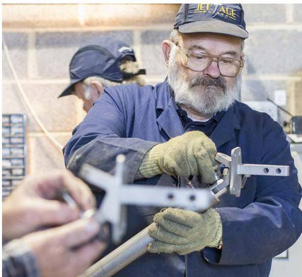
Renishaw produced the unconventional brackets for the cockpit using the latest metal additive manufacturing technology, allowing the Typhoon restoration project to continue as planned.
