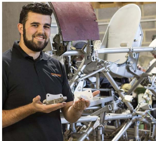
Renishaw produced the metal brackets from aluminium powder in four separate builds using one of its AM250 additive manufacturing machines.
